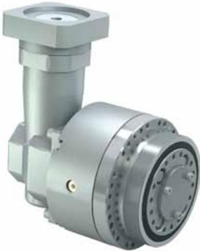
High precision reduction gear with possibility of right-angle motor connection also allows increasing of total reduction ratio using a input right-angle reducer. This allows using of a servomotor with a lower power and higher speed i.e., smaller motor. This solution is available for whole E type series reduction gears.
